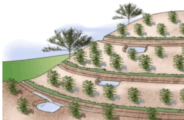
Figure 20: Terracing along contours to minimize rainwater runoff
